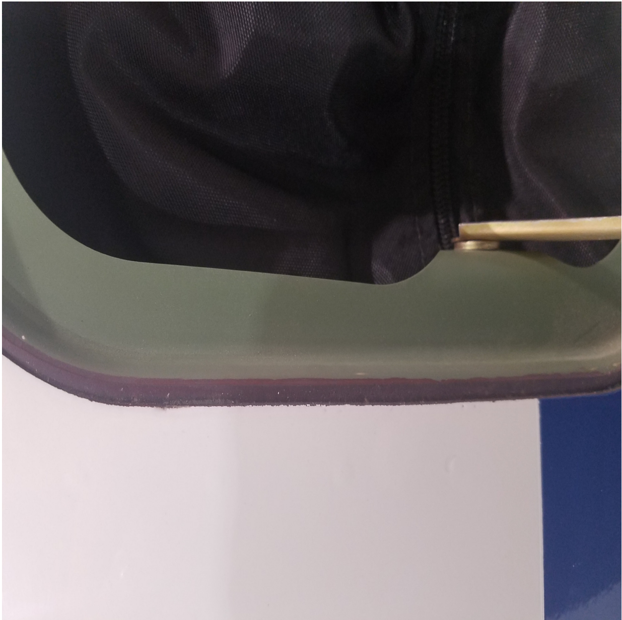
Figure 1, Sheet 2. Acceptable, No Over-spray
